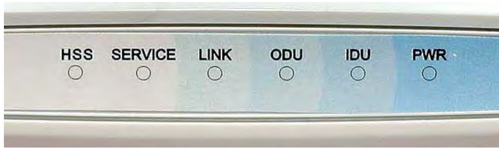
Figure 3-14: IDU-E Front Panel LEDs
