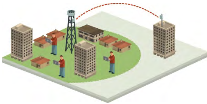
Figure 1-3: Typical WiFi Backhaul Application
