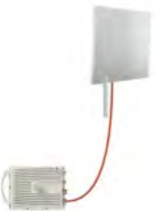
Figure 17-7: Incorrectly mounted ODU (No “water nose”)
