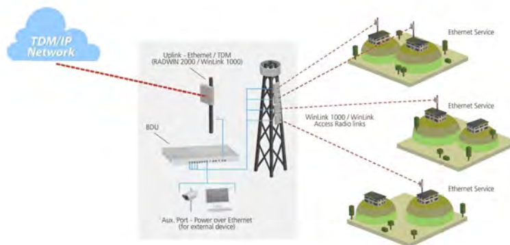
Figure 1-21: Typical Multiple Point-to-Point deployment with wireless uplink
