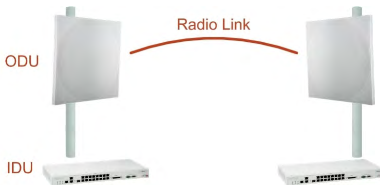
Figure 1-7: Example of Link Architecture - System Components
