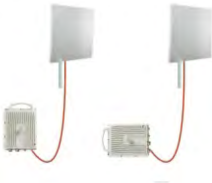
Figure 17-6: Mounted ODUs with correct “water nose”
